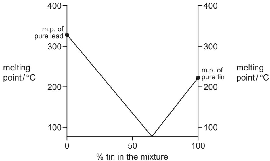
The graph shows that any mixture of lead and tin must have a melting point that is
