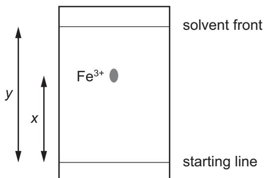
To make the spot containing  $\text{Fe}^{3+}(\text{aq})$  more visible, the paper is sprayed with aqueous sodium hydroxide so that a precipitate of iron(III) hydroxide forms.
